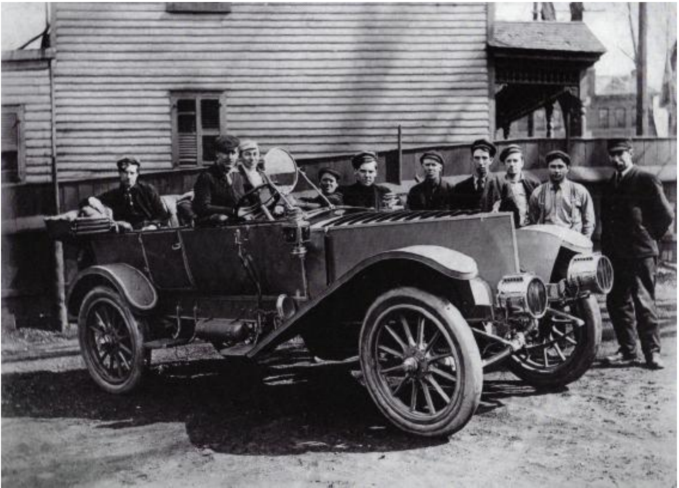
In honor of Franklin car owner and lover, MMUUS member Hank Manwell, this is a photo of a special model that executive H. H. Franklin had built for himself in 1909. His nickname for it was the "Torpedo." It had no radiator, but used air vents on top of the hood for cooling purposes.
